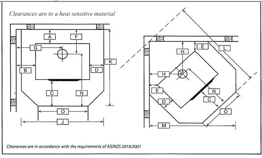
When installing the Firenzo fire on a leg base ADD 70mm to vertical measurements shown:
